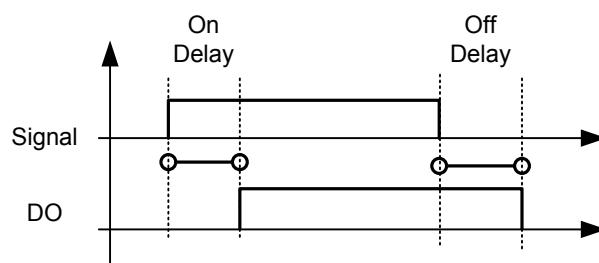
*Figure 22. Digital outputs 1 and 2, on- and off-delays*
