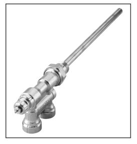
The RA 15/6T and TB is a special conversion valve that allows a single connection point-at the side of the radiator- to serve as both the supply & return for a hot water based system. An example of its application is the transformation of a 1-pipe steam system into a hot water based system.
