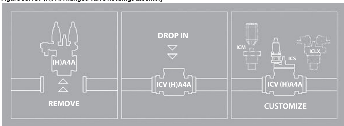
Figure 53: ICV (H)A4A flanged valve housings assembly
