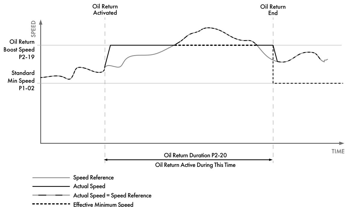
If the drive run command is removed whilst the oil-return feature is active, the drive will follow the selected ramps to a stop and normal operation will commence on next start. The only deviation from this would be if the minimum on time set in the drive had not yet been observed, and the drive would continue to operate as indicated above until the minimum on time had been observed.
