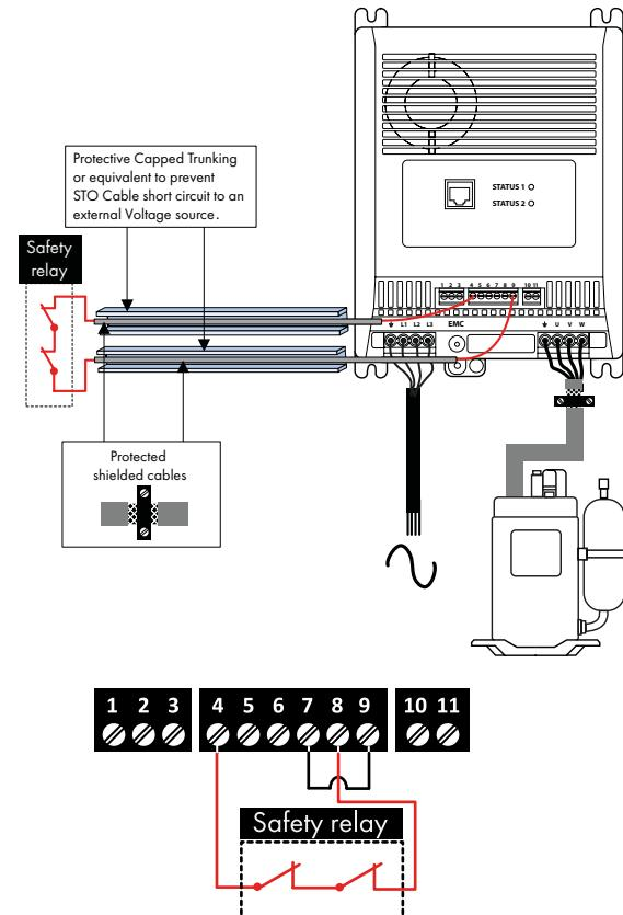
**NOTE** The Maximum cable length from Voltage source to the drive terminals should not exceed 25 metres.
