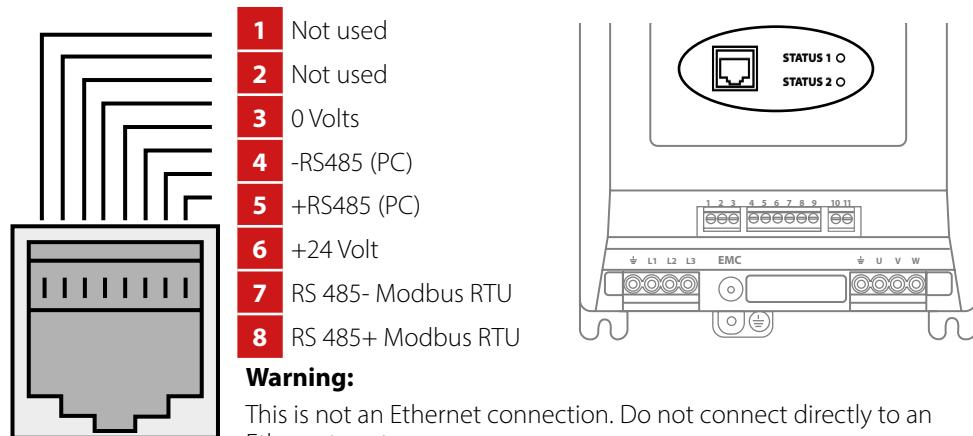
The RJ45 port has some terminals that are internally connected in parallel with the pluggable control terminals as shown below:
