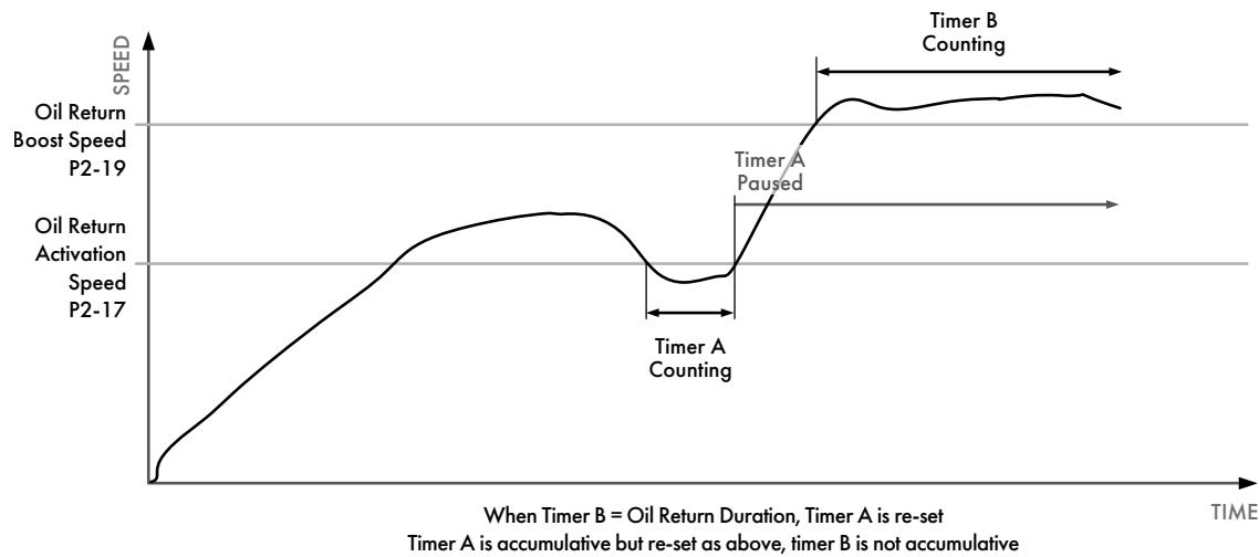
When the timer is re-set (Timer A), the minimum speed clamp is returned to the value set in P1-02 and P2-19 is ignored until the next activation of the Oil Return Feature.
