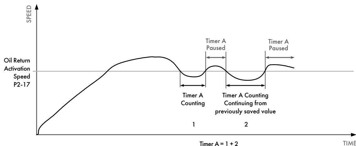
The above illustrates that the timer will count when the speed is below the activation speed and the value in the timer will be held and used the next time that the speed falls below the activation speed – this is a cumulative timer.
