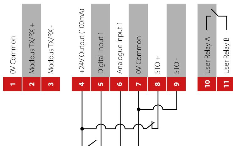
STO signal must be provided in order to permit running the motor. Start/Stop command provided by the Digital Input. The speed reference is provided by the output of the PI controller and the PI feedback is provided by the analogue input. The drive can be re-set from a fault by removing and re-applying the digital input.
