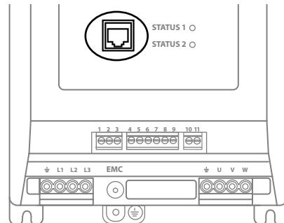
The RJ45 port has some terminals that are internally connected in parallel with the pluggable control terminals as shown below:
