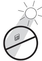
The installation height should be 1,5 m minimum from the floor surface. The room sensor needs to be at least 0,5m away from doors and windows.
