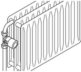
Direct heat radiation from large radiators may disturb the Radiator Thermostats ability to measure the room temperature correctly.
