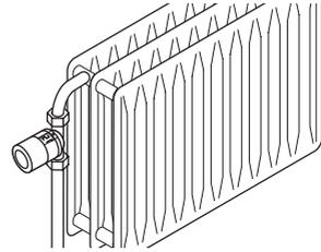
To avoid this, mount the thermostat pointing away from the radiator. The optimal solution is a Radiator Thermostat with a Danfoss Ally™ Room Sensor.
