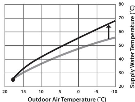
*NOTE: If system is installed during period with outside temperature > 10°C opening point will not be found until temperature drops below 7-8°C.0*
