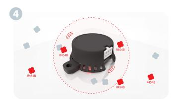
By controlling the current to the heating element, the thermal response of the temperature sensor will depend on the thermal conductivity of the gas present in the gap between the heating element and the temperature sensor.
