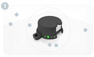
The TC sensor uses the thermal transfer properties of gases as a measurement tool for the presence of gas. The thermal conductivity of gases is inversely proportional to molecular weight. Therefore, thermal conductivity decreases with increasing molecular weight.
