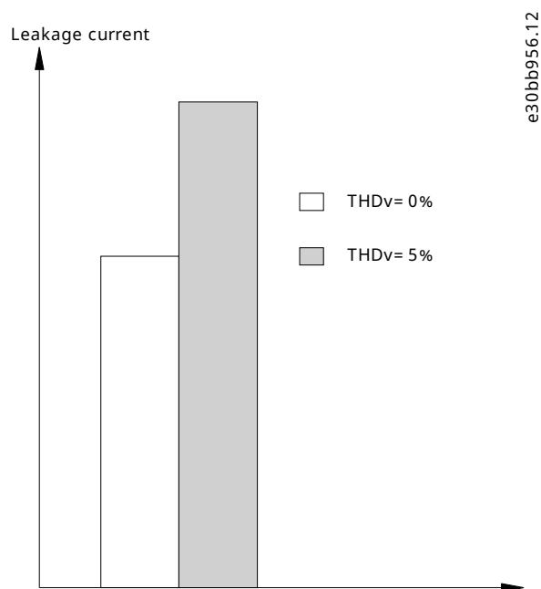
Figure 29: Line Distortion Influences Leakage Current
