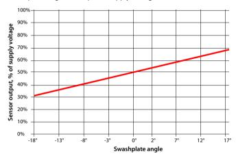
Swashplate angle vs. output of supply voltage
