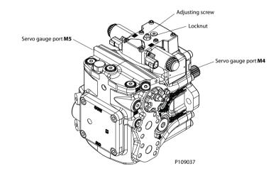
**4.** Rotate the neutral adjusting screw clockwise until the pressure increases on the gauge. Note the angular position of the wrench. Then rotate the neutral adjusting screw counter clockwise until the pressure increases by an equal amount on the other gauge. Again note the angular position of the wrench.
