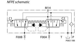
The pump displacement is proportional to the solenoid signal current, but it also depends upon pump input speed and system pressure. This characteristic also provides a power limiting function by reducing the pump swashplate angle as system pressure increases. A typical response characteristic is shown in the accompanying graph. Under some circumstances, such as contamination, the control spool could stick and cause the pump to stay at some displacement.
