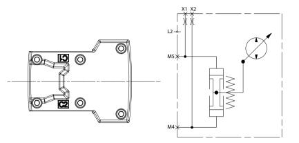
Pump flow direction with NFPH control
