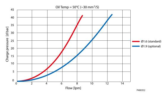
When a pump is used with an external loop flushing shuttle valve, ensure that the charge setting of the pump matches the setting of the loop flushing shuttle valve. Contact your Danfoss representative for the availability of additional charge relief settings.
