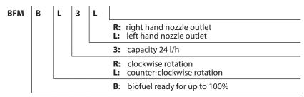
Nozzle capacity at 4.3 cSt., 10 bar, 2800 min<sup>-1</sup>
