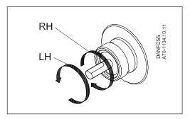
Note! Shaft rotation, location of nozzle outlet and other connections are seen from shaft end.
