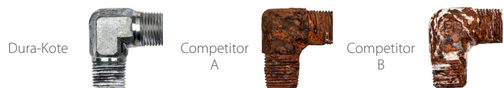
Corrosion comparison after 650 hours of exposure to salt spray testing.
