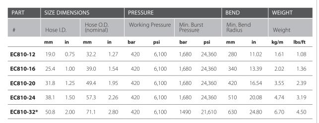
\* With the 6S fitting the -32 size working pressure is 350 bar (5100 psi) with a 4:1 safety factor.
