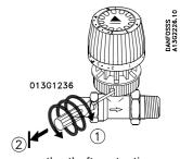
To remove the theft protection use screwdriver 013G1236 and screw into the hole (1). Pull out until the stop is reached (2).
