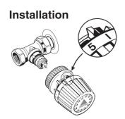
Remove the valve cover. Check that the thermostat is set at the factory setting of 5.
