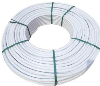
The white Danfoss FH composite pipe is 100% impervious to air, temperature resistant and highly flexible. It consists of an aluminum pipe which is covered inside and out with a Polyethylene (PE-RT) layer. All layers are permanently bonded with each other through a layer of adhesive.
