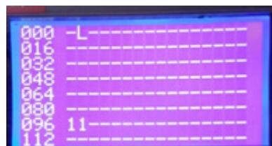
The two 1-digits represent the addresses 96 (HP module) and 97 (Receiver module) respectively.
