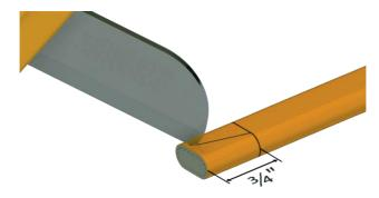
• Remove the exposed grounding braid. Make sure that the insulation jacket is not damaged.
