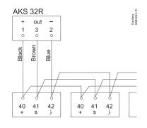
The signal from one pressure transmitter can be received by up to 10 controllers.
