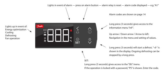
Shows the setting for a chosen parameter / saves a changed setting. Short press gives access to entering of the thermostat's cut-out limit.
