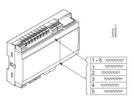
The controller is provided with labels from the factory indicating a generic application. When selecting the required application, specific labels are provided so that you can mount the relevant one.
