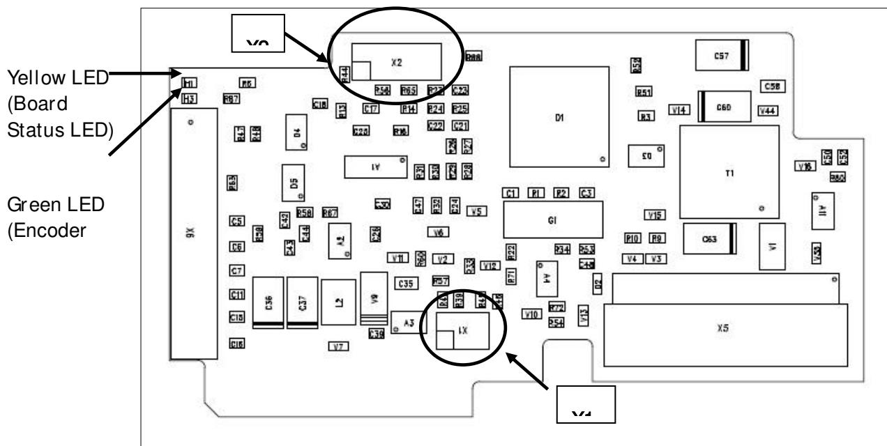
**Description:** Encoder board for **VACON® NXP** with an input for *EnDat/SSI* absolute encoder and *Sin/Cos* type encoder.
