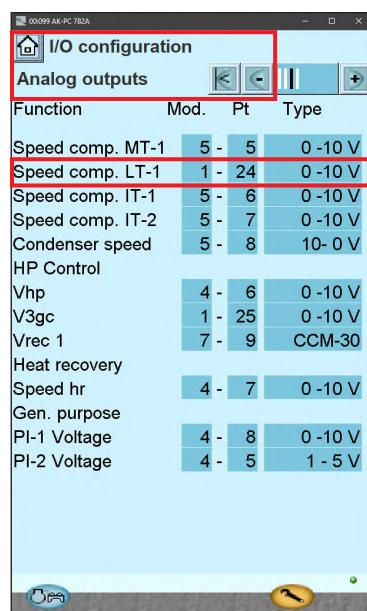
'Speed comp. LT-1 AO' is wired directly to 'PI-2 in voltage' AI created in next step.
