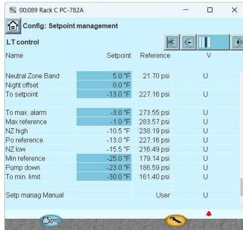
Neutral zone band = this setting straddles to setpoint setting to determine when to activate and deactivate compressor stages. Inverter is used to stay within neutral zone.
