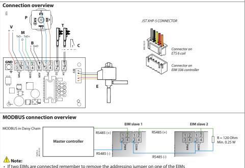
MODBUS transmission lines usually require termination resistors, especially for longer cable lengths
