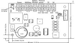
A Note: S2 - Temperature sensor S4 - Temperature sensor or DI Weight: 40 gm
