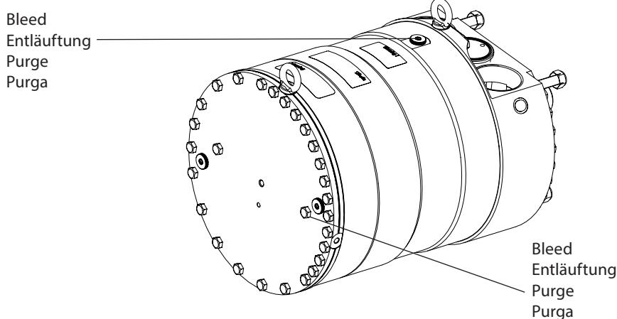
The bleeding kit makes it possible to bleed a pump from a distance. The hose can be cut in the preferred length and makes it possible to direct the water from bleeding back to drain or holding tank.
