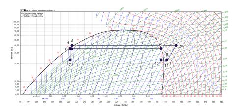
At 50 bar high pressure the discharge temperature is 55 °C and therefore it is possible to start reclaiming heat from the system but there is no temperature difference of the heat exchanger.
