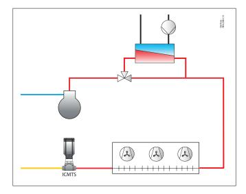
Under these conditions the discharge temperature from the compressors is approx 35  $^{\circ}$ C and therefore it is not possible to make 55  $^{\circ}$ C hot water.
