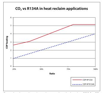
From the chart above it can be seen that the heating COP for  $CO_2$  is from approx 25 % to 150 % better that R134A and best at part load which is the main part of the year.
