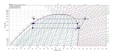
At 80 bar approx 80 % of the heat is reclaimed at a cooling COP of 3.13. To increase the ratio to more than 80 % the pressure can be pushed up and the gas cooler can be by-passed.
