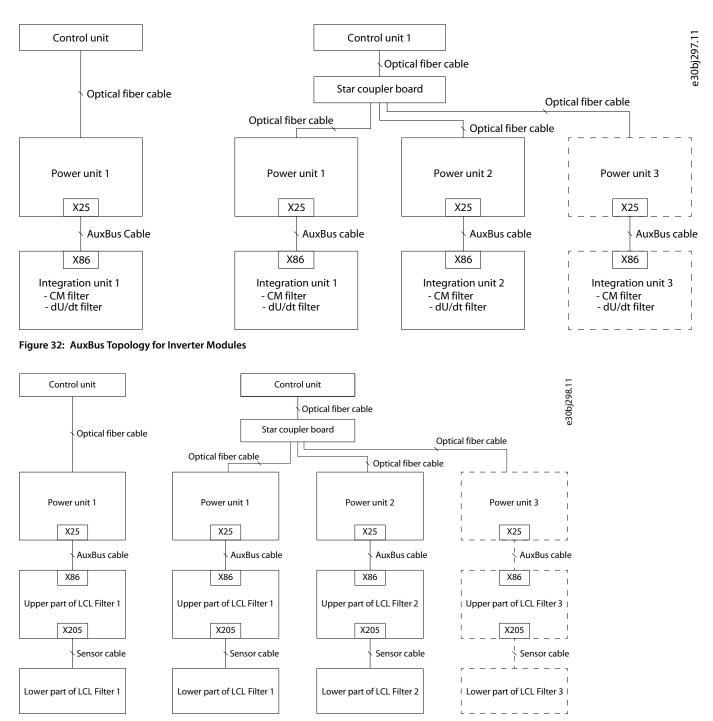
Figure 33: AuxBus Topology for AFE Modules and LCL Filters
