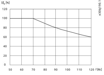
Figure 37: Output Frequency Derating
