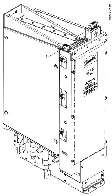
Figure 35: AuxBus Terminals of the LCL Filter
