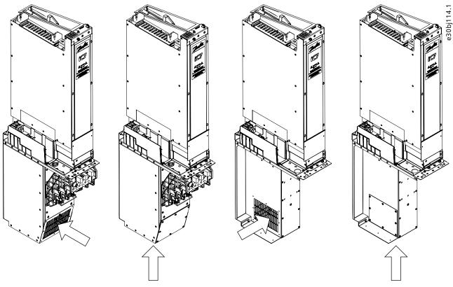
Figure 12: Inlet Airflow from the Front or from Below
