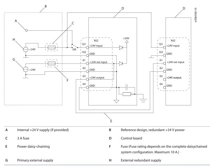
Figure 101: Wiring Diagram of Redundant Supplies
