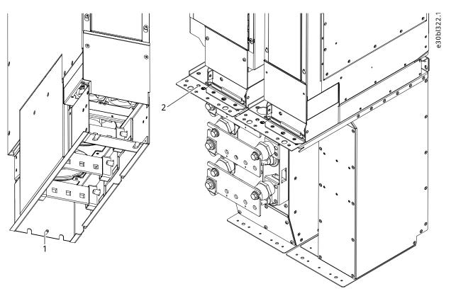
Figure 17: Grounding Stud of the Inverter Module and Grounding Terminal of the LCL Filter
