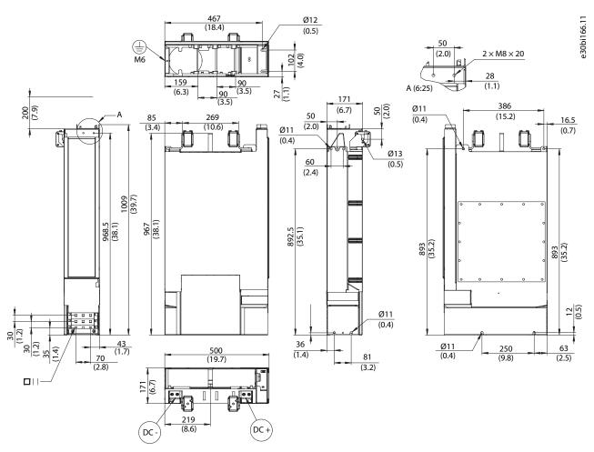
Figure 61: Dimensions of the Inverter Module in mm (in), IM10
