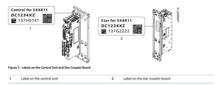
There are similar identification labels on the integration units, filters, and other components. For example, the LCL Filter has a power unit label, like on the system modules. The integration units have an identification label that shows to which system module it belongs.
