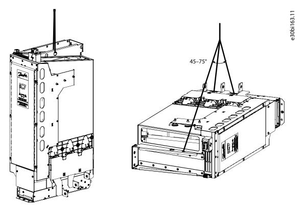
Figure 3: Lifting the Upper Part of the LCL Filter, AFE
