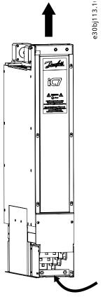
Figure 11: Cooling of System Modules without Integration Units
