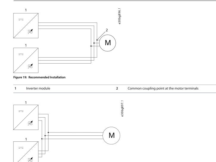
Figure 20: Alternative Installation Method
