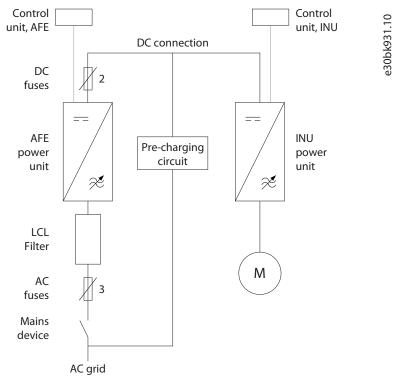
Figure 27: DC Connections of Single Power Units
