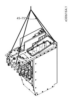
Figure 4: Lifting the Integration Unit
