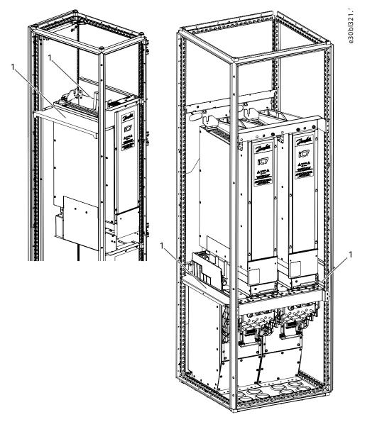
Figure 14: Air Guides of the IM10/IM11 (left) or IR10/IR11 (right) Modules in the Cabinet
