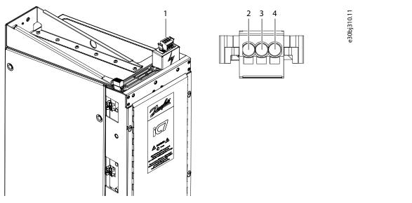
Figure 21: Fan Supply Connector of the LCL Filter
