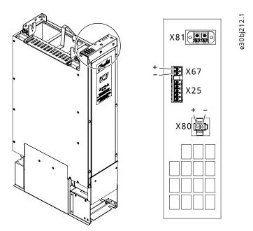
Figure 31: Auxiliary Connections of the Power Unit
