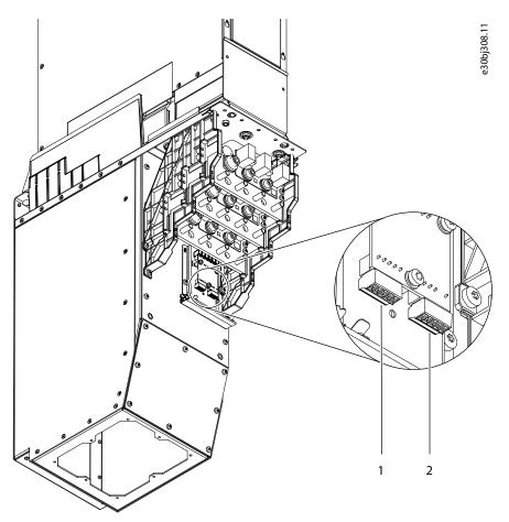
Figure 36: AuxBus Terminals of the Integration Unit
