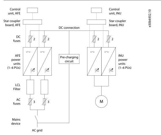
Figure 28: DC Connections of Parallel Power Units
