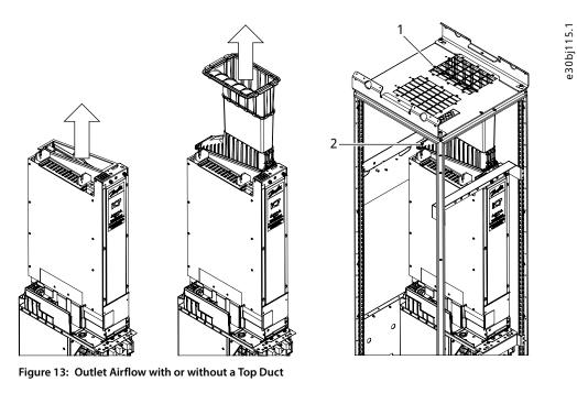
1Top duct mounted to roof of cabinet2Top duct mounted to back wall of cabinet
