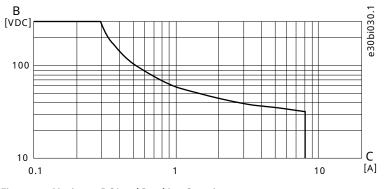
Figure 47: Maximum DC Load Breaking Capacity
