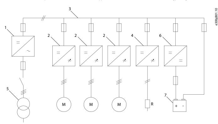
Figure 5: An Example of a Common DC Bus Drive System
