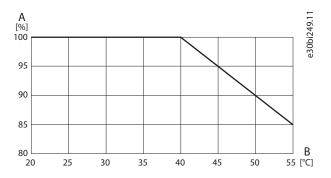
Figure 103: Output Current Derating vs. Ambient Temperature
