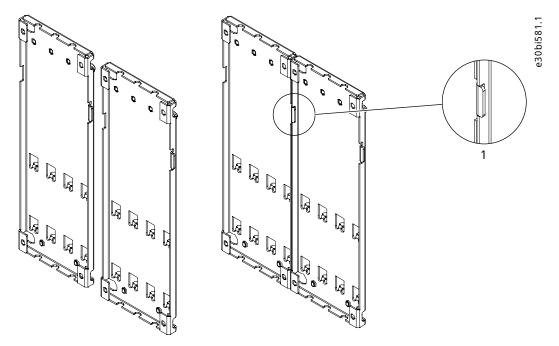
Figure 49: Attaching Mounting Plates to Each Other
