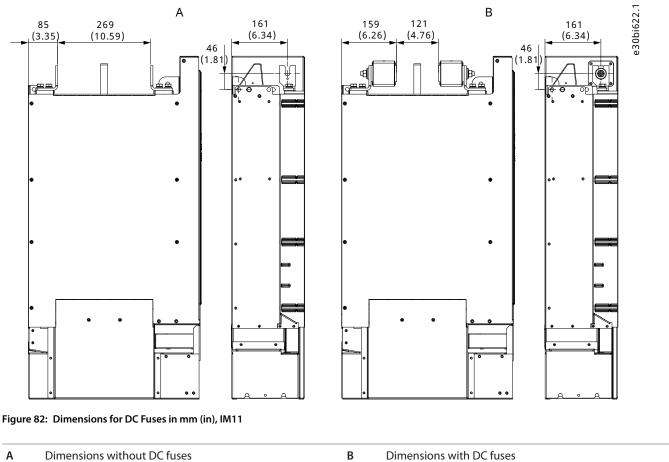
Α Dimensions without DC fuses Dimensions with DC fuses
