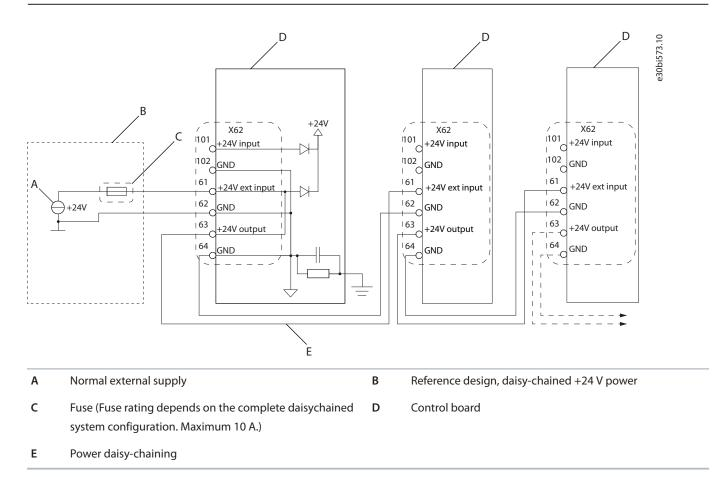
Figure 102: Wiring Diagram of a Daisy-chained +24 V Supply for the Control Units
