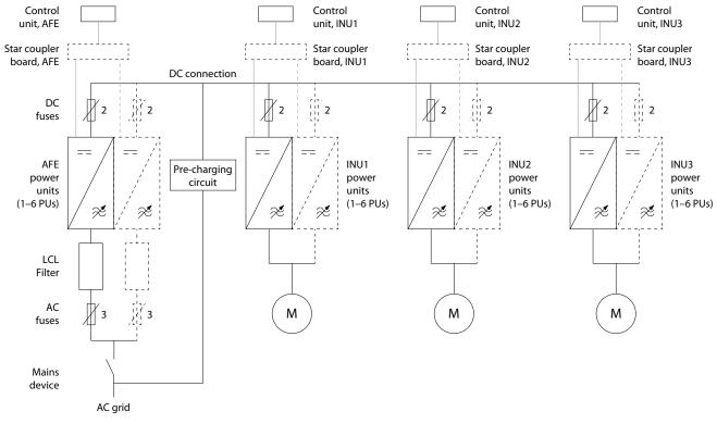
Figure 29: DC Connections of a Drive Lineup
