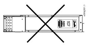
Figure 10: Forbidden Installation Direction of the Inverter Module
