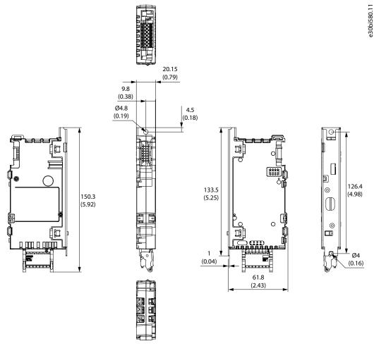
Figure 91: Dimensions of an Option Board in mm (in)
