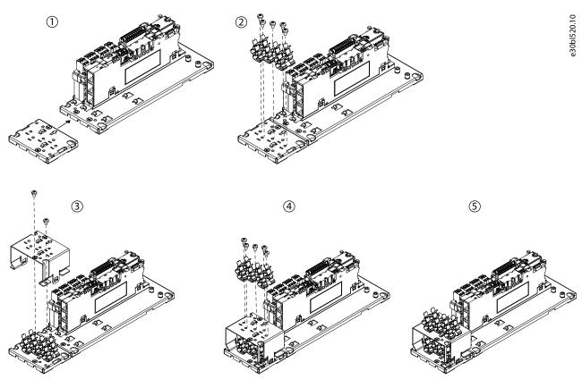
Figure 48: Assembling the Mounting Plate
