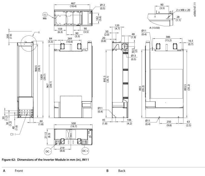
C The front fixing beam can be rotated so that the screws can be attached from the front or from the top.
