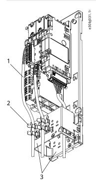
Figure 52: Example of Installing the Control Cables
