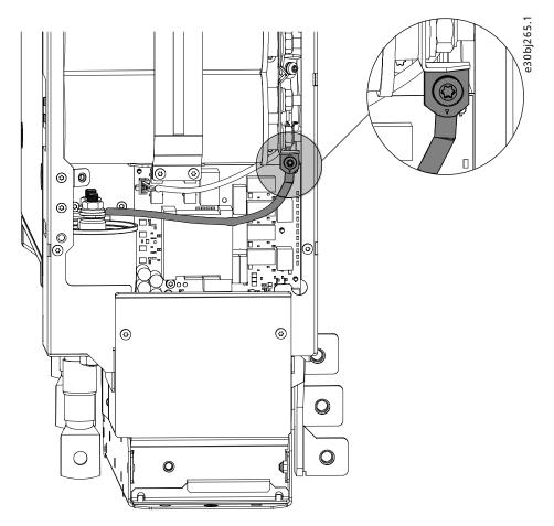
Figure 25: EMC Protection Level 3
