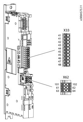
Figure 41: Control Board Terminal Block and Terminal Numbering
