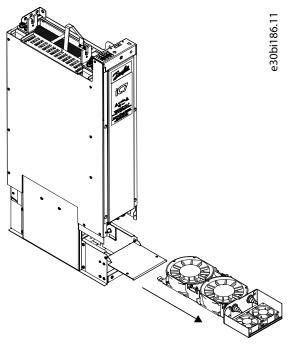
Figure 60: Removing the Fan Assembly
