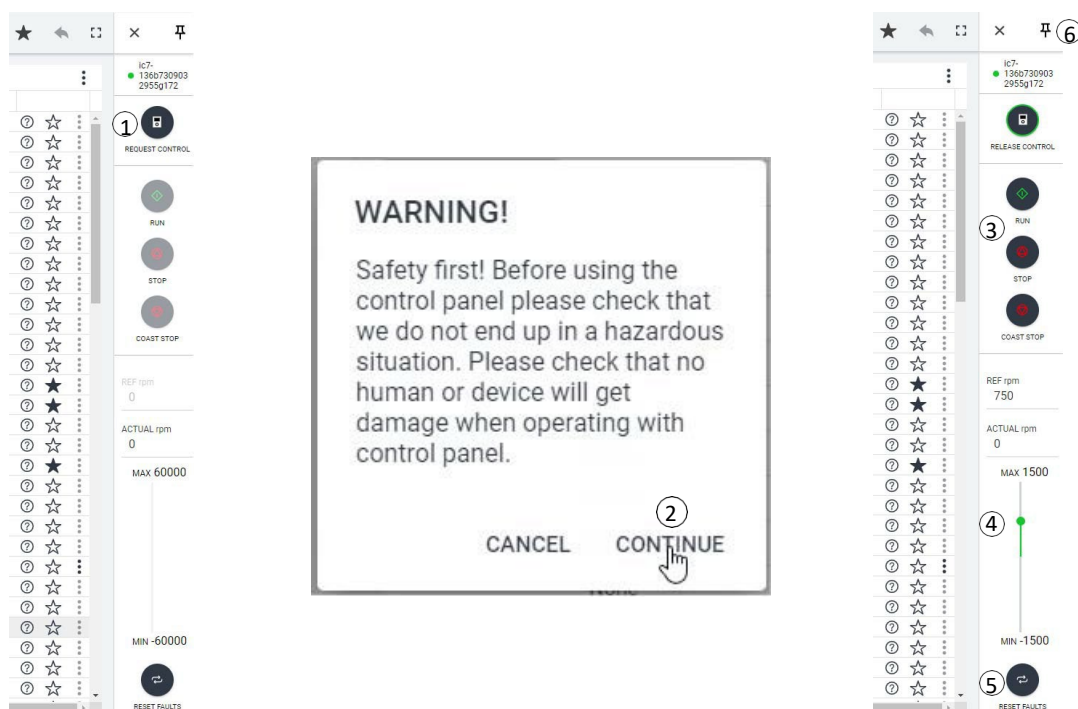
Figure 27: Operating the drive with MyDrive® Insight
