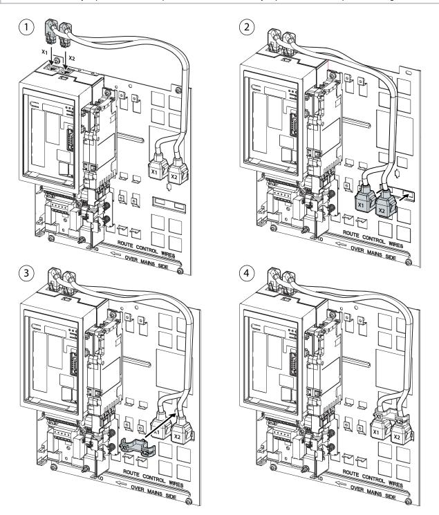
Figure 2: X1 and X2 Jumper Cable Installation on Control Board Mounting Plate
