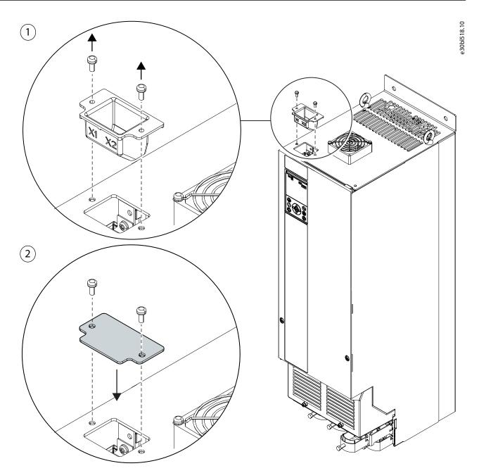
Figure 1: Top Cover Plate Installation
