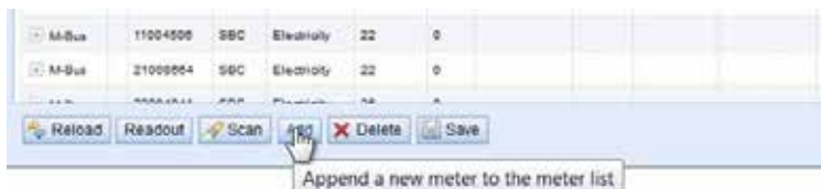
Figure 19: Adding a meter manually in tab Meter
