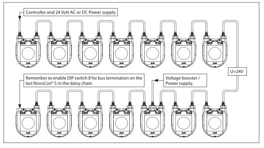
NovoCon® S with temperature sensors and Voltage booster/ Power supply.
