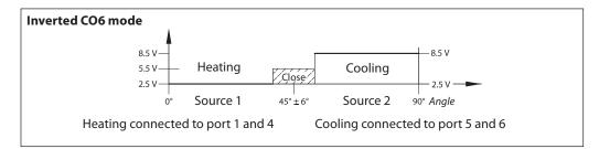
Signal from NovoCon® S to the Actuator NovoCon® ChangeOver<sup>6</sup>
