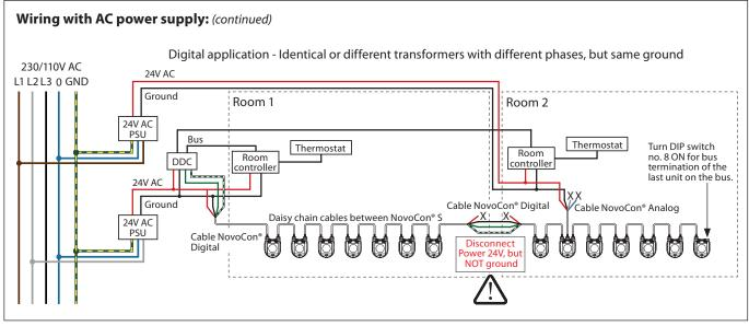
Wires that ends in an "X" must be properly terminated.
