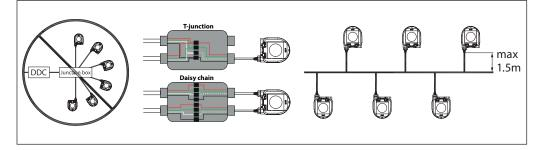
If the supply voltage to the first device in the daisy chain is lower than 24V AC/DC, or long thin cables other than NovoCon<sup>®</sup> cables are used, then the quantity of devices in the daisy chain may have to be reduced.
