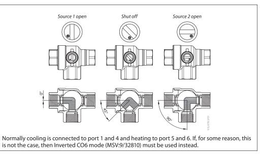
CO6, contrary to other ball valves, includes a shut off function. This function should only be used during maintenance and not during operation. This replaces the need for four ball valves.
