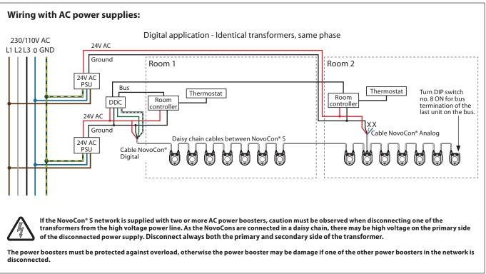
Wires that ends in an "X" must be properly terminated.
