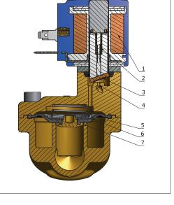
1. Coil 2. Armature spring 3. Armature 4. Pilot orifice
