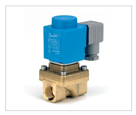
EV250B with assisted lift can operate from zero and up to 10 bar differential pressure. This 2/2-way valve program is especially to use in closed circuits with low differential pressure, but demanding moderate flow rates. Valve body in dezincification resistant brass for ensuring a long life even in connection with aggressive steam media. EV250B is compatible with the broad Danfoss coil program with enclosures from IP00 up to IP67. Medium temperatures up to 140 °C (low pressure steam).
