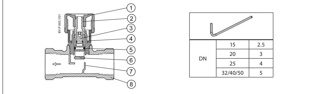
ASV-I incorporates a double cone able to give maximum stroke limitation, thus achieving flow limitation. It also incorporates shut off function. ASV-I is equipped with the nipples for the flow measurement and a connection for the ASV-I/ ASV-PV impulse tube.
