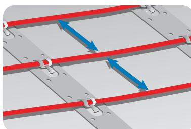
$$C - C [cm] = \frac{\text{Površina [m}^2\text{]}}{\text{Duljina kabela [m]}} \times 100 \text{ cm}$$
