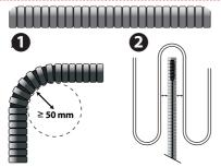
The sensor should be mounted in an insulating conduit, sealed at the end, for easy replacement of the sensor if required.
