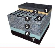
1. Top layer of concrete slab or asphalt concrete.
