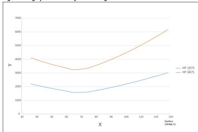
Χ Inlet pressure HP side [Bar] Υ Mass flow HP side [kg/hr]
