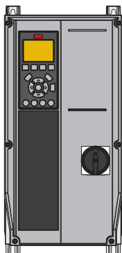
A4 IP55 with mains disconnect
