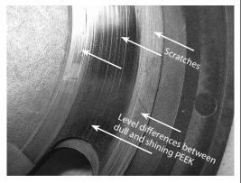
If the port plate has scratches, level differences or both between the arrows, the port plate must be replaced.
