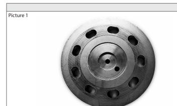
A normally worn valve plate has no marks/scratches but only a slightly polished surface.
