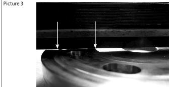
A good way to identify a worn valve plate is to hold a straight knife edge over the valve plate. When holding it up to the light, it will be possible to see any space between the knife edge and the valve plate. See picture 3.
