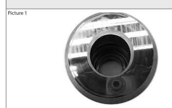
If the swash plate is polished 360°, it is an indication of insufficient filtration.
