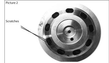
A worn valve plate has scratches, and/or a polished surface. Even small scratches will give a loss of flow.
