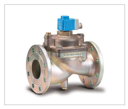
EV220B 65 - EV220B 100 is a 2/2-way solenoid valve program for use in robust industrial applications, demanding high flow rates. The valve is designed with cast iron valve body and flanged connection.
