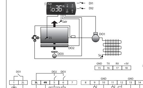
Note: 2L and 3L must be connected to the same phase.
