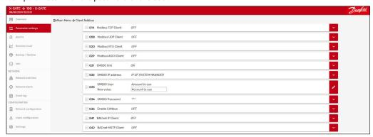
After this configuration done, X-Gate will start to automatically collect data from the System Manager and automatically will create all the CDF files of the discovered devices (nodes) and create the related device in the Network Configuration page.
