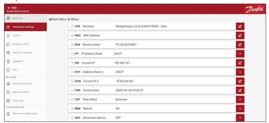
In case of STATIC IP management, set up parameters **IP1** & **IP21** to "Static". **BBB** parameter can be used in case of manual reboot of the X-Gate machine.
