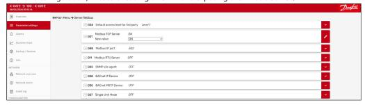
In case of sharing data with a local BMS, the full list of variable/data-points can be downloaded as a CVS file with the utility in settings  $\rightarrow$  download CSV file.
