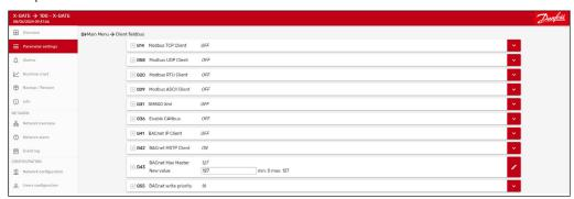
After this configuration done, X-Gate will start to automatically scan the network (IP or Serial as per configuration done) and automatically will create all the CDF files of the discovered devices (nodes) and create the related device in the Network Configuration page.
