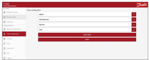
All the Accounts has a dedicated profile to have different visibility inside the X-Gate configuration page. Profiles available are **Maintenance** and **Service**.
