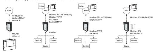
X-Gate can provide flexibility with focus on 3rd party device integration into System Manager and at the same time make easy for a BMS to integrate the desired data-points over standard protocols.
