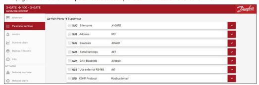
SU2 & SU3 are the configuration parameters for the serial line at COM1.
