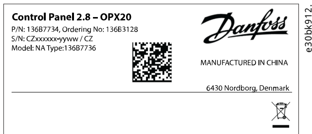
Figure 56: Example of a Control Panel Label
