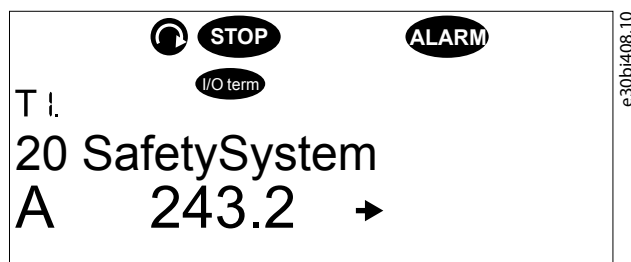
Illustration 76: Fault Presentation in the Fault Lists. The Source and Fault Number Are Shown as "source.number" (instead of "T1->T16" for Other Faults).
