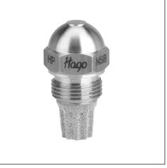
Many nozzles are satisfactory for spraying liquids, but for a positive cut-off ask for the Hago type 4023 nozzle. Our exclusive design produces a precisely controlled flow rate and spray angle and includes a liquid cut-off near the orifice. Fluid cut-off near the orifice can be very important in situations where excessive after drip can damage or destroy things located beneath the nozzle.
