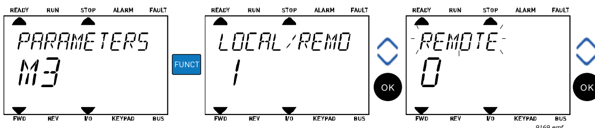
Figure 24. Changing control places
