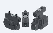
DG valves mount on industry standard surfaces and provide 3 or 4-way control in a broad range of applications, industrial and mobile. Their primary function is to direct fluid flow to a cylinder or to control the direction of rotation of a hydraulic motor. These valves can be actuated by solenoid, hydraulic or pneumatic pilot, lever, or mechanically.
