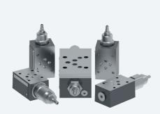
These compact hydraulic systems feature modular valves that are "sandwich" mounted between a directional control valve and a standard mounting surface. All circuit flow paths are contained within the control valve and modules. These valves provide a compact hydraulic circuit at a reduced cost, eliminating interconnecting piping. Each valve "stack" can be configured to provide the specific system functions.
