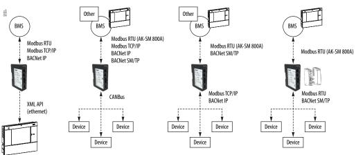
X-Gate can provide flexibility with focus on 3rd party device integration into System Manager and at the same time make easy for a BMS to integrate the desired data-points over standard protocols.
