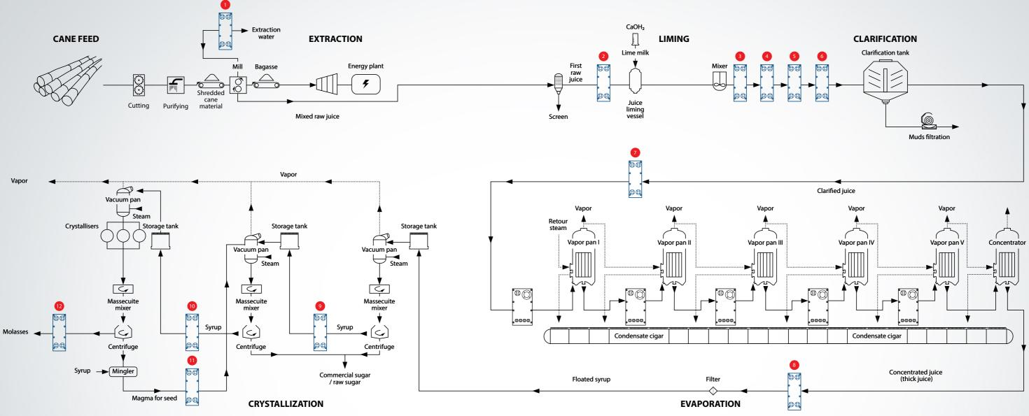
The cane is delivered to the mill, where it is cut, cleaned (purified), and transferred to the mill. Here, the cane is cut into pieces with revolving knives, shredders, or crushers (for breaking down the organic material) and then ground (or milled) in a series of roller mills (consisting of 3-6 rollers each), being transported from one mill to the next.
