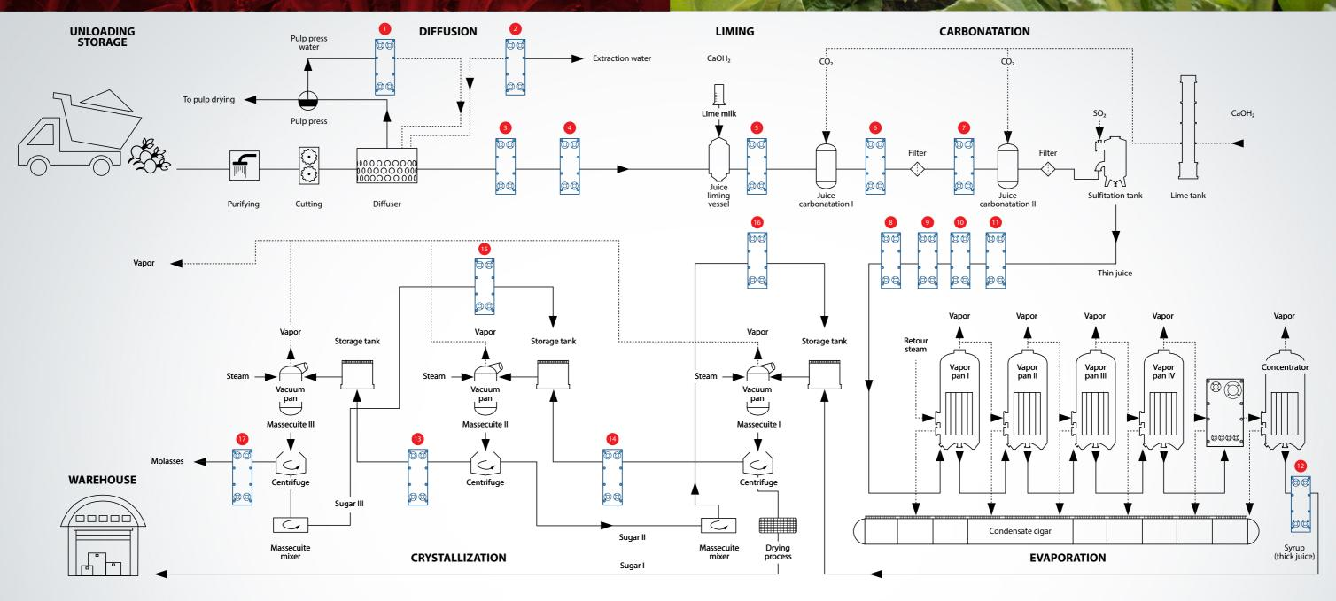
Nowadays, a diffusion method is usually applied for obtaining beet juice. The first step in the diffusion process is to cut the beet roots into thin strips called cossettes. The cossettes then undergo countercurrent processing with hot water at temperatures of 72-75°C in a special machine referred to as a diffuser.
