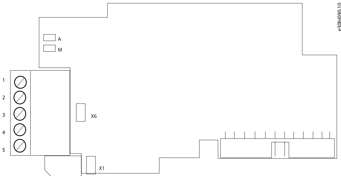
Illustration 35: The OPTC6 Option Board Layout
