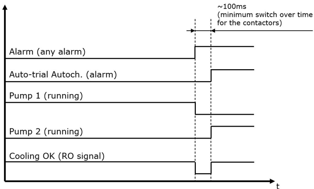
Figure 8. Response of the auto trial function to an alarm
