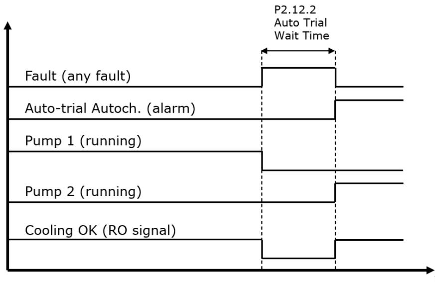
Figure 9. Response of the auto trial function to a fault
