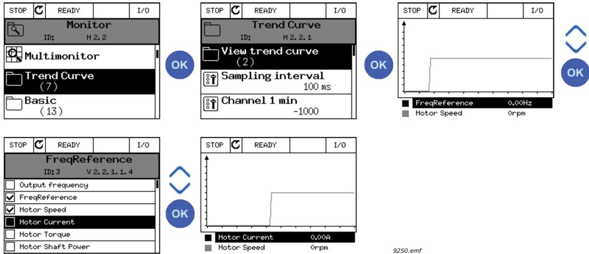
The Trend Curve feature also allows you to halt the progression of the curve and read the exact individual values.
