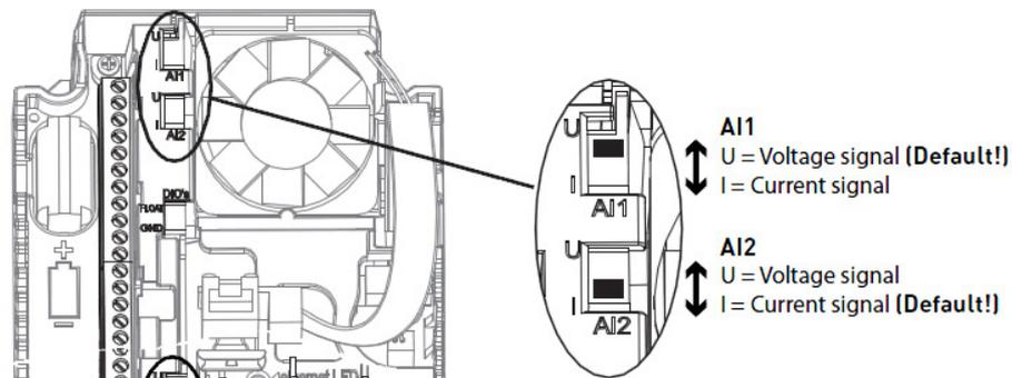
**Note!** If you are using signal range 4..20 mA or 2..10V, set the analog input DIP switch according to signal type (voltage or current) and select “4..20mA/2..10V” signal range by analog input signal range –parameter in corresponding parameter P2.3.3.1 AO Range Sel.(2V/4mA).
