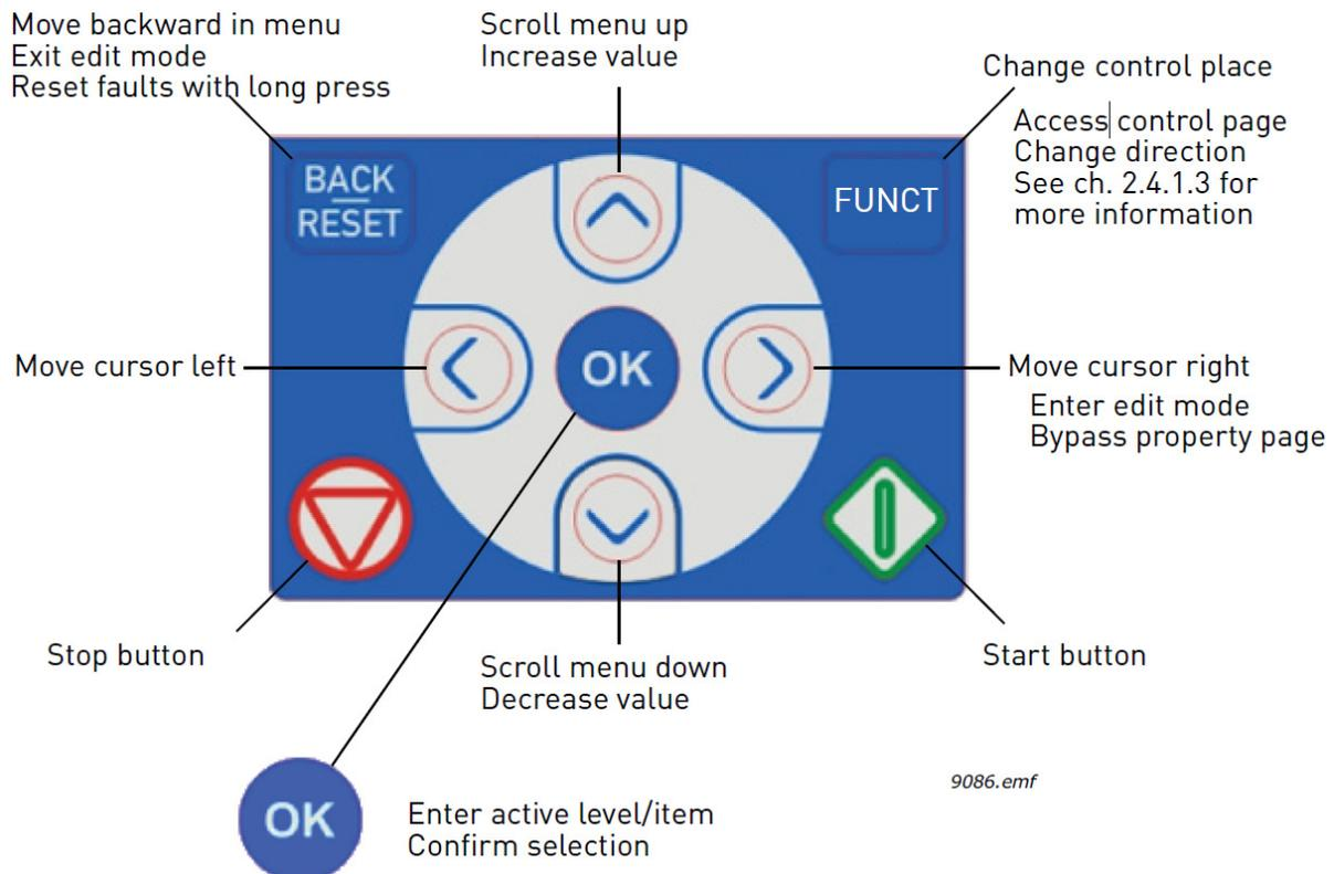
The data on the control panel are arranged in menus and submenus. Use the Up and Down arrows to move between the menus. Enter the group/item by pressing the OK-button and return to the former level by pressing the BACK/RESET-button.
