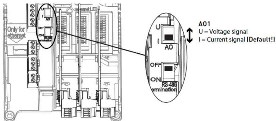
**Note!** If you are using signal range 4..20 mA or 2..10V, set the analog input DIP switch according to signal type (voltage or current) and select “4..20mA/2..10V” signal range by analog input signal range –parameter in corresponding parameter P2.3.3.1 AO Range Sel.(2V/4mA).
