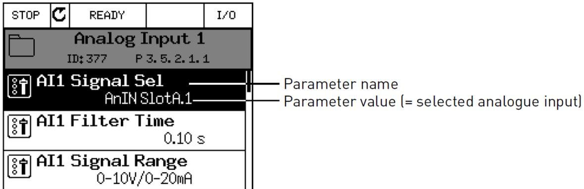
Given the standard I/O board compilation on the VACON® 100 control unit, there are 2 analog inputs available (Slot A terminals 2/3 and 4/5). In the programming view, these inputs are referred to as follows:
