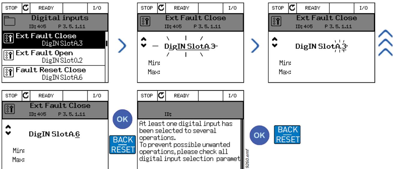
Figure Error! No text of specified style in document.6. Programming digital inputs with keypad
