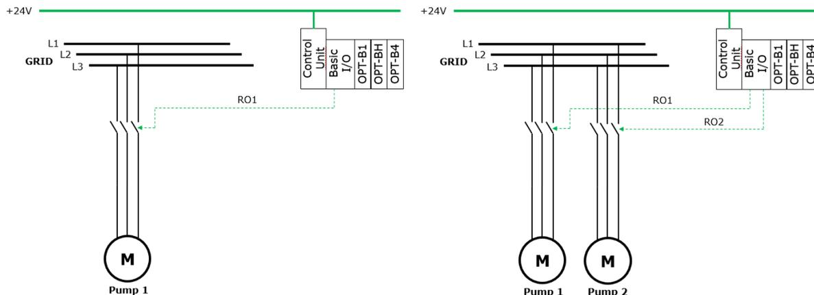
Figure 1. Cooling unit configurations (1 and 2 pump systems)
