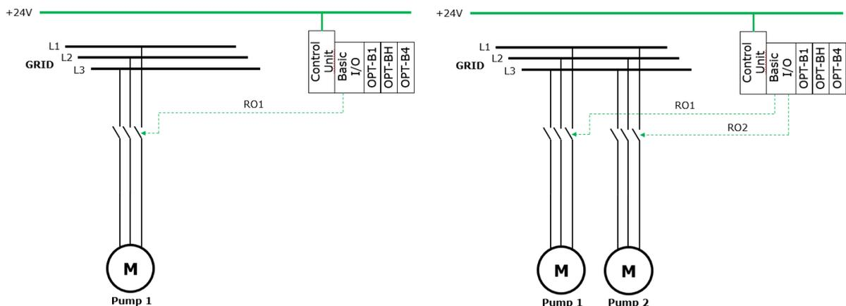
Figure 3. Different configurations of iC7 Series Cooling Module
