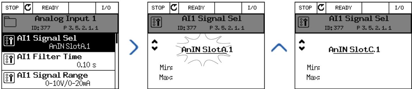
Figure 7. Programming analog input signal with graphical LCP
