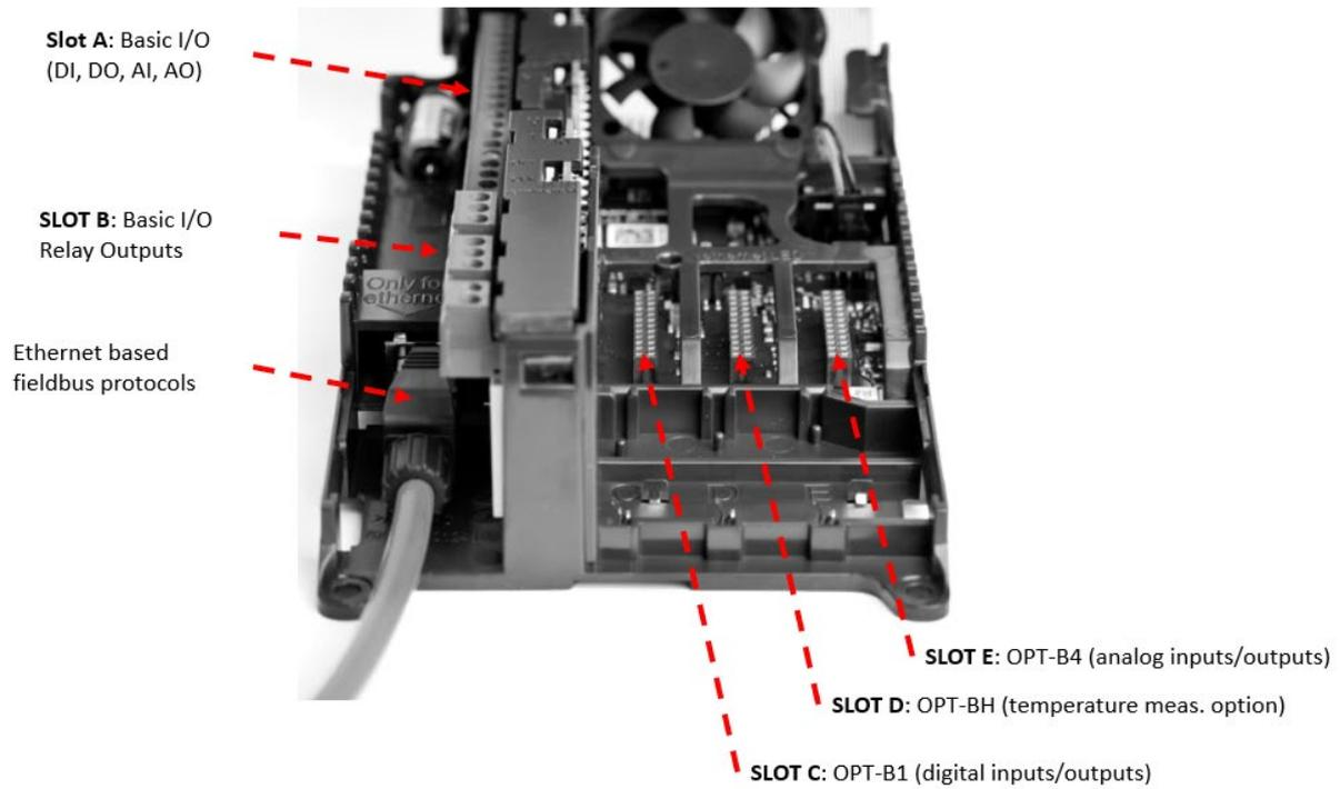
Figure 2. Control unit and option boards
