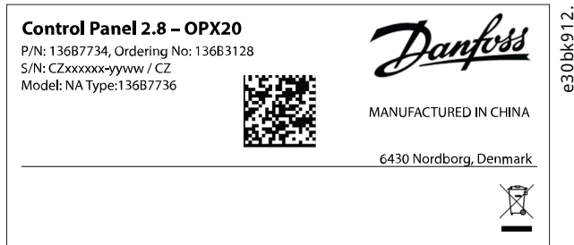
Figure 56: Example of a Control Panel Label
