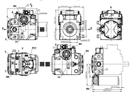
**A/B** system ports: Ø31.5 mm; M12 x 1.75; 20 min. full thread depth **MA/MB** (system), **M3** (charge) gauge ports per ISO 11926-1:  ${}^{9}\!\!/_{16}$ –18 **M4, M5** (servo), **M14** (case) gauge ports per ISO 11926-1:  ${}^{7}\!\!/_{16}$ –20 **L2, L4** – Case drain ports per ISO 11926-1:  ${}^{15}\!\!/_{16}$ –12
